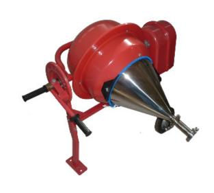
The Original Extraction Contraption harnesses the sub-zero temperatures of dry ice sublimation along with centrifugal force to produce plant essence in a fraction of the time of traditional processes. There is no water or harsh chemicals used during the extraction process. In fact, our process actually removes much of the plant's natural moisture. The final essence is a fine, dry powder.
